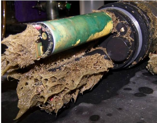
*Figure 1. Water quality sonde with soft fouling*
