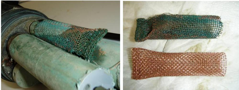
Figure 4. Anti-fouling copper “sock” used for conductivity sensors
