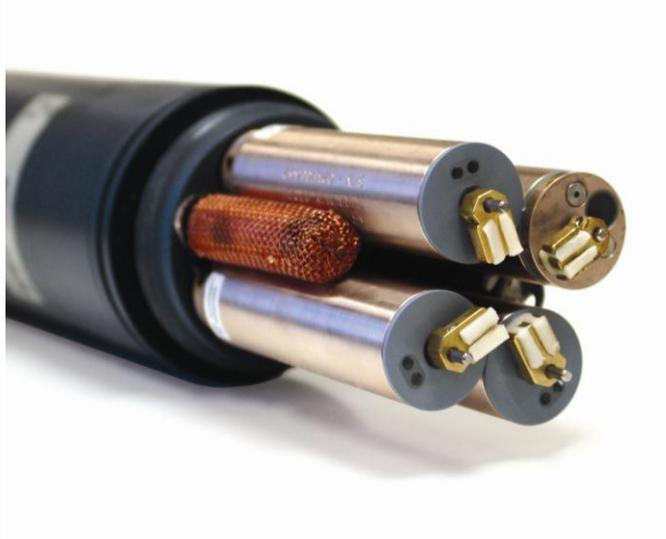
*Figure 13. YSI water quality probes with copper-alloy housings and wipers. The conductivity/temperature probe has been treated with C-Spray coating and copper screen*
