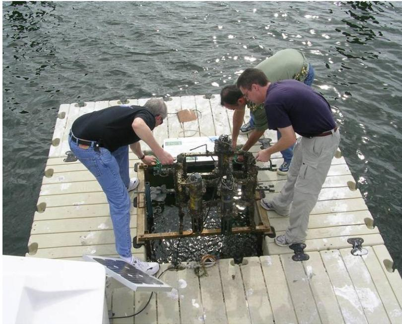
*Figure 3. Test platform in St. Petersburg Harbor used for anti-fouling testing*
