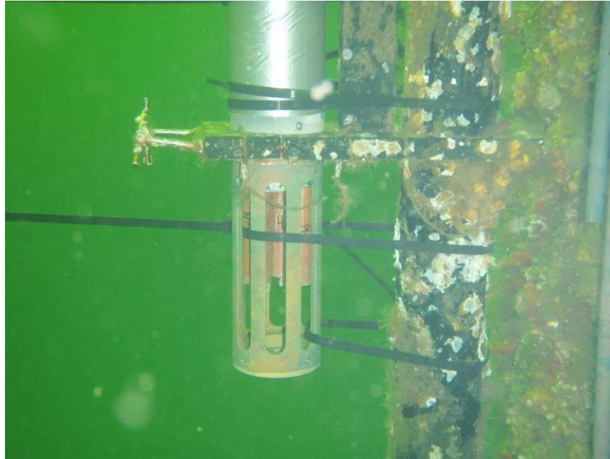
Figure 10. Sonde deployed with anti-fouling kit in Gulf of Mexico. Copper-alloy parts are extremely resistant to fouling, often going 10 months before cleaning is required.
