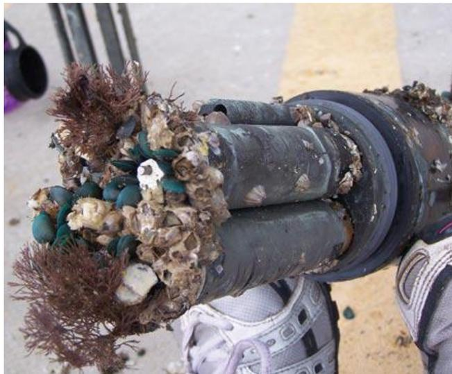
*Figure 2. Water quality sonde with hard fouling*
