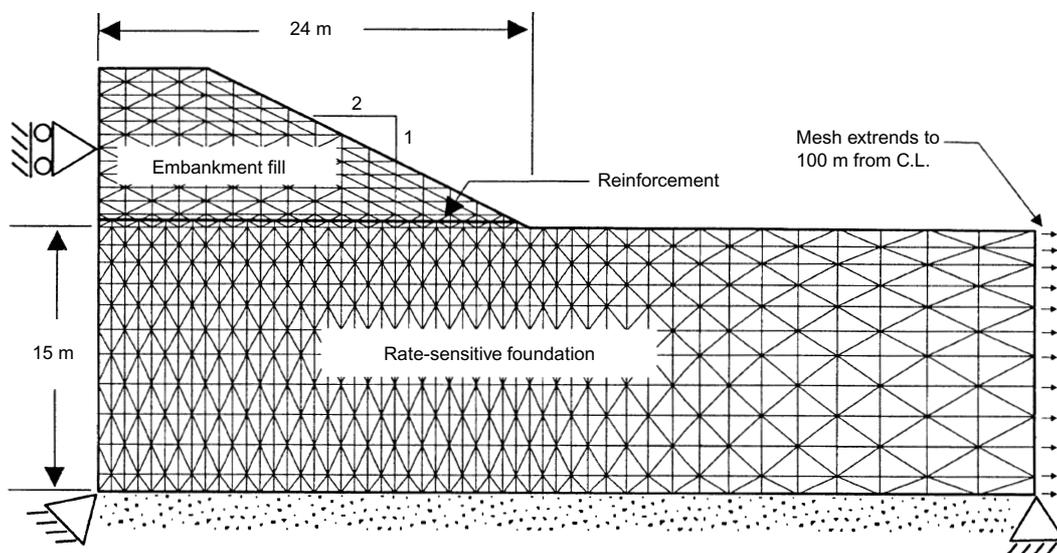
Fig. 1. The finite element mesh and geometry of the system
