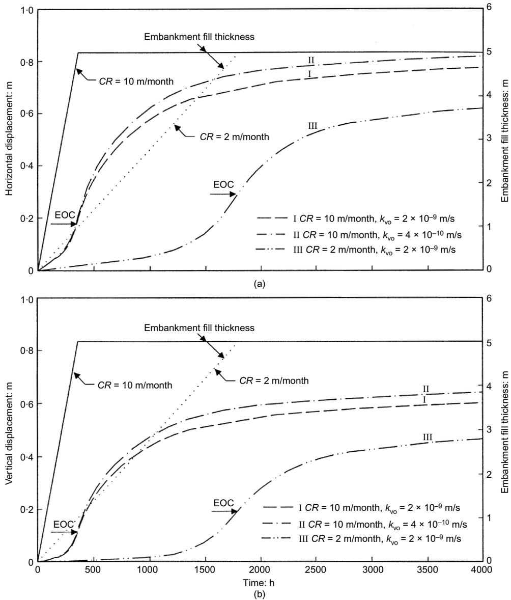
Fig. 9. Deformations at the toe for embankments over soil C-R1 ( $H = 5$  m,  $J = 2000$  kN/m): (a) horizontal deformations; (b) heave
