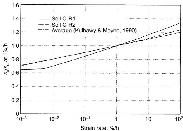
Fig. 4. The effect of strain rate on the undrained shear strength,  $s_u$ , of soils C-R1 and C-R2
