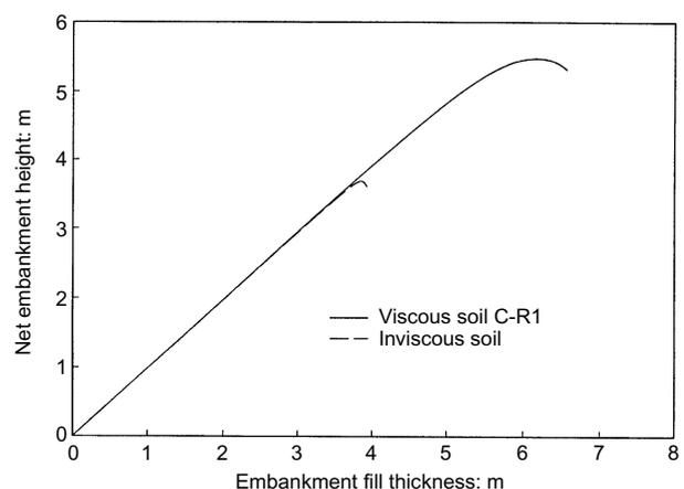
Fig. 5. The variation of net embankment height with fill thickness for the unreinforced embankment with  $CR = 10$  m/month
