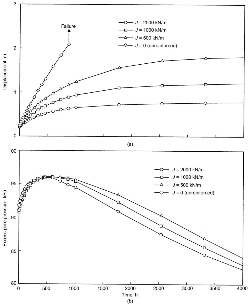
Fig. 12. Effect of reinforcement on pore pressure and creep deformations for cases with  $H = 5$  m,  $CR = 10$  m/month and soil C-R1 with  $k_{v0} = 2 \times 10^{-9}$  m/s: (a) horizontal toe deformation; (b) pore pressure at location 4.8 m deep and 6.8 m away from centreline
