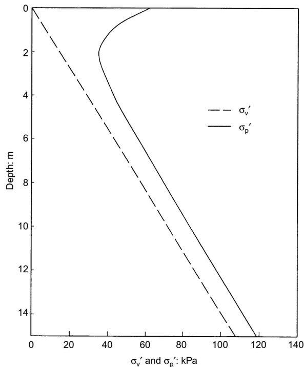
Fig. 3. Initial vertical effective stress and preconsolidation pressure profiles for both soils C-R1 and C-R2
