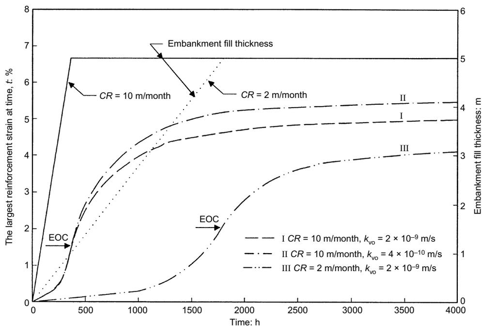
Fig. 7. Reinforcement strains developed for embankments over soil C-R1 ( $H = 5$  m,  $J = 2000$  kN/m)
