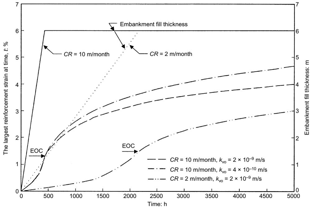
Fig. 8. Reinforcement strains developed for embankments over soil C-R2 ( $H = 6$  m,  $J = 2000$  kN/m)
