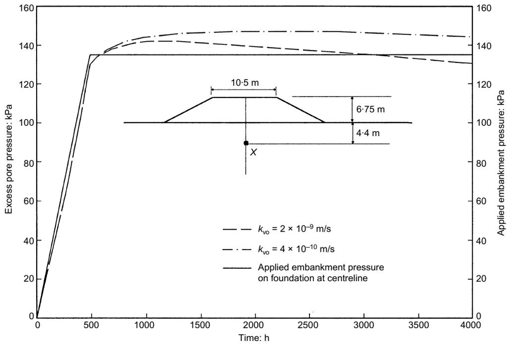
Fig. 10. Maximum excess pore pressure at point X in the foundation soil C-R1 for cases with  $H = 6.75 \text{ m}$ ,  $CR = 10 \text{ m/month}$  and  $J = 2000 \text{ kN/m}$
