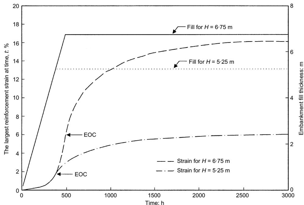
Fig. 6. Reinforcement strain developed during the short term for embankments with  $CR = 10$  m/month,  $J = 2000$  kN/m over soil C-R1
