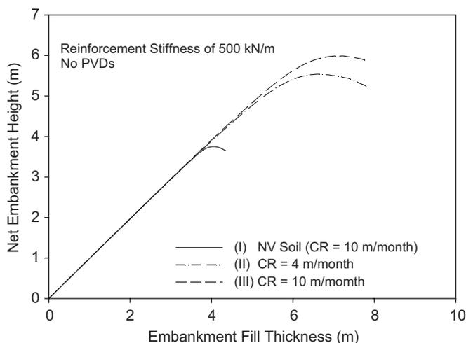
Fig. 4. Effects of rate-sensitivity and construction rate on the short-term embankment failure height.
