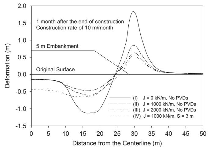
Fig. 12. Effect of reinforcement stiffness and PVDs on the differential settlement of the foundation surface.
