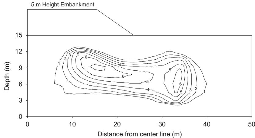
Fig. 10. The difference of excess pore water contour at the end of construction and 1 month after the end of construction (CR = 10 m/month,  $J = 2000 \text{ kN/m}$ ).
