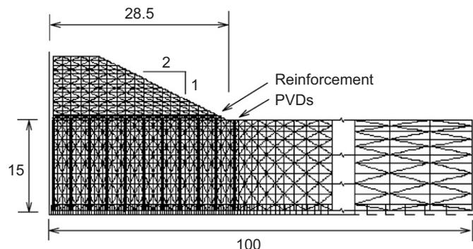
Fig. 1. Finite element mesh discretization.
