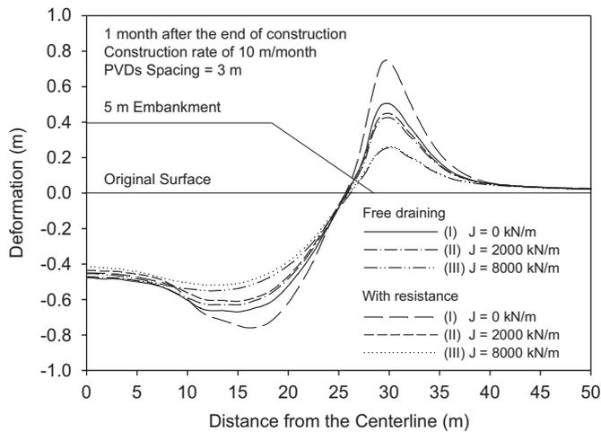
Fig. 14. Effect of assumptions regarding resistance to drainage in the PVDs on the differential settlement at the foundation surface.
