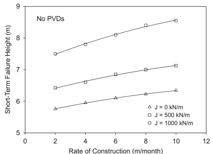
Fig. 5. Effects of reinforcement stiffness and construction rate on the short-term embankment failure height.
