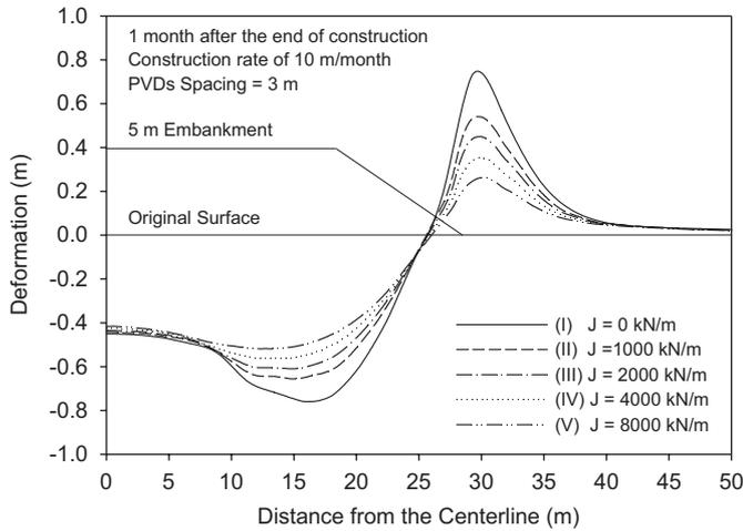
Fig. 13. Effect of reinforcement stiffness on the differential settlement of the foundation (PVDs at 3 m spacing for all cases).
