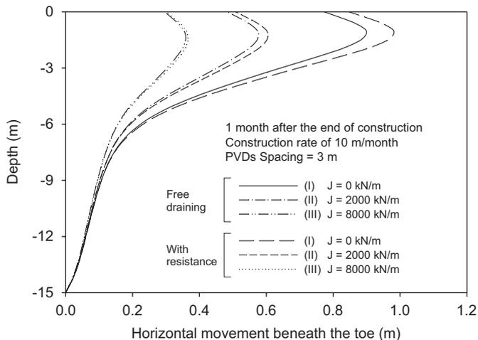
Fig. 17. Effect of assumptions regarding resistance to drainage in the PVDs on horizontal deformations beneath the embankment toe.
