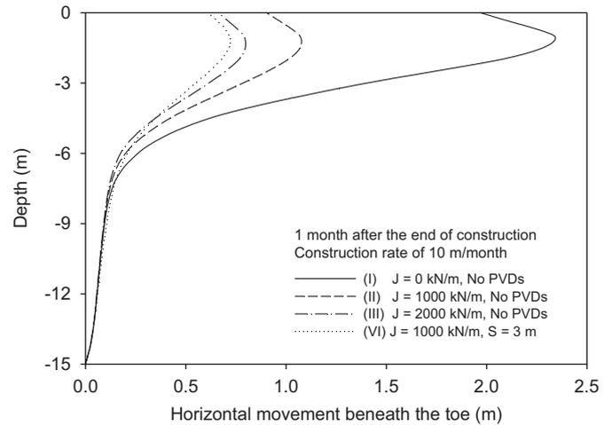
Fig. 15. Effect of reinforcement stiffness and PVDs on the horizontal deformation beneath the embankment toe.
