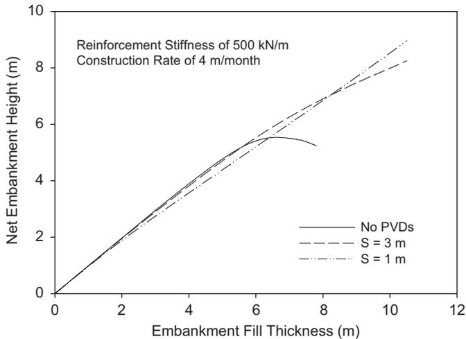
Fig. 6. Effect of PVDs on short-term embankment failure height.
