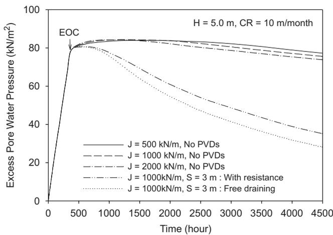
Fig. 11. Effect of reinforcement stiffness and PVDs on the dissipation of excess pore pressure with time at the location of the maximum difference shown in Fig. 10 (i.e. 6 m beneath the embankment shoulder).
