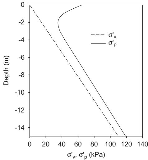
Fig. 3. Preconsolidation pressure and initial vertical stress profiles (based on Rowe and Li (2002)).
