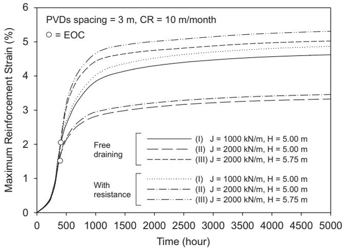
Fig. 8. Effects of PVDs and reinforcement stiffness on the mobilization of reinforcement strain with time.
