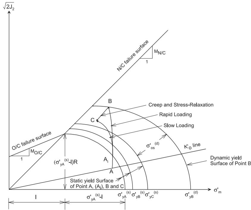
Fig. 2. Elliptical cap model (modified from Rowe and Hinchberger (1998)).
