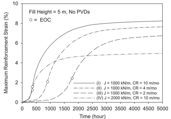
Fig. 7. Effects of construction rate and reinforcement stiffness on the maximum mobilized reinforcement strain with time.
