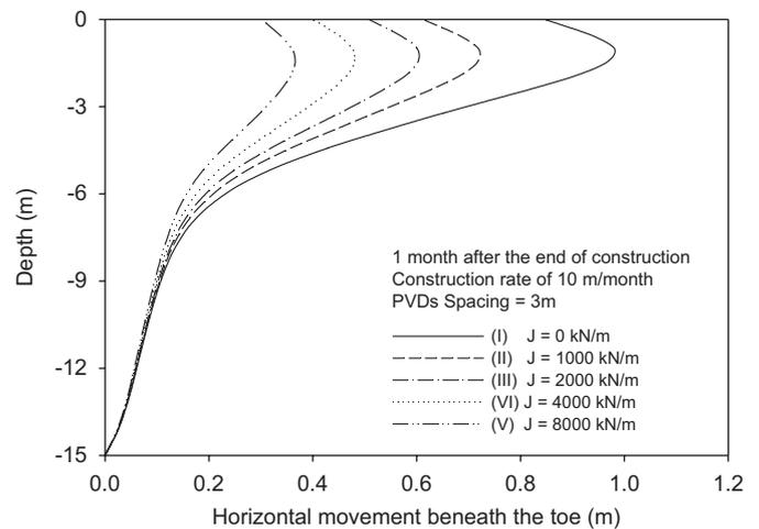
Fig. 16. Effect of reinforcement stiffness on horizontal deformation beneath the embankment toe (PVDs at 3 m spacing for all cases).
