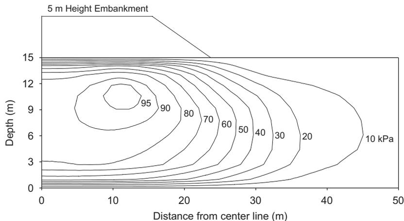
Fig. 9. Contours of excess pore water pressures 1 month after the end of construction (CR = 10 m/month,  $J = 2000 \text{ kN/m}$ ).
