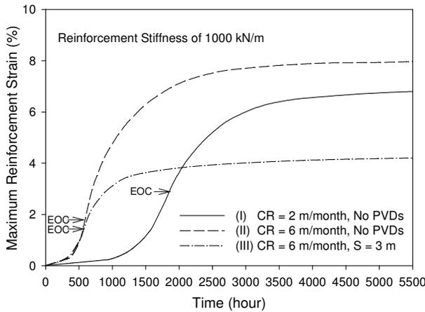
Figure 5. The effect of construction rate and PVDs on the long-term mobilized reinforcement strain
