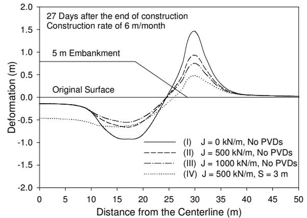
Figure 6. The effect reinforcement stiffness and PVDs on differential settlement
