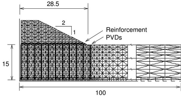
Figure 1. Finite elements mesh discretisation.
