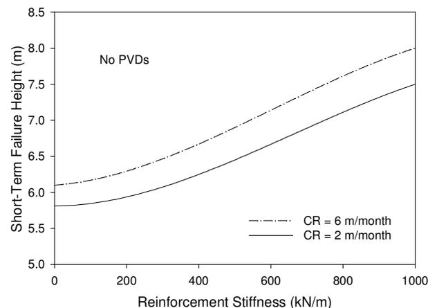
Figure 3. The effect of reinforcement stiffness on the short-term embankment stability
