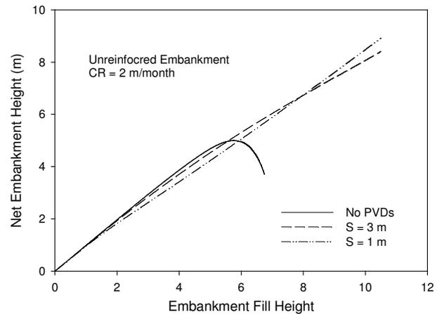
Figure 4. The effect of PVDs on the short-term embankment stability
