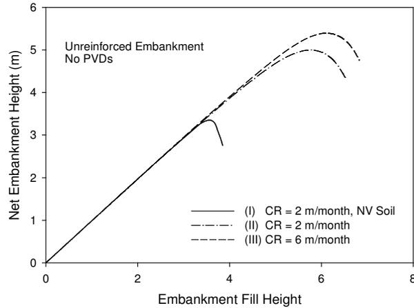
Figure 2. The effect of soil viscosity and construction rate on the short-term embankment stability
