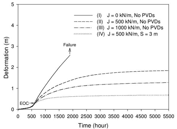
Figure 7. The effect reinforcement stiffness and PVDs on the lateral deformation at the embankment toe
