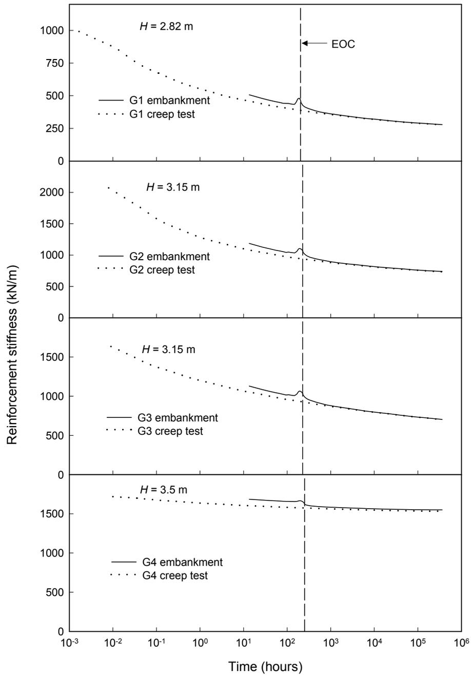
Figure 10. The variation of reinforcement stiffness with time for embankments over Soil A.
