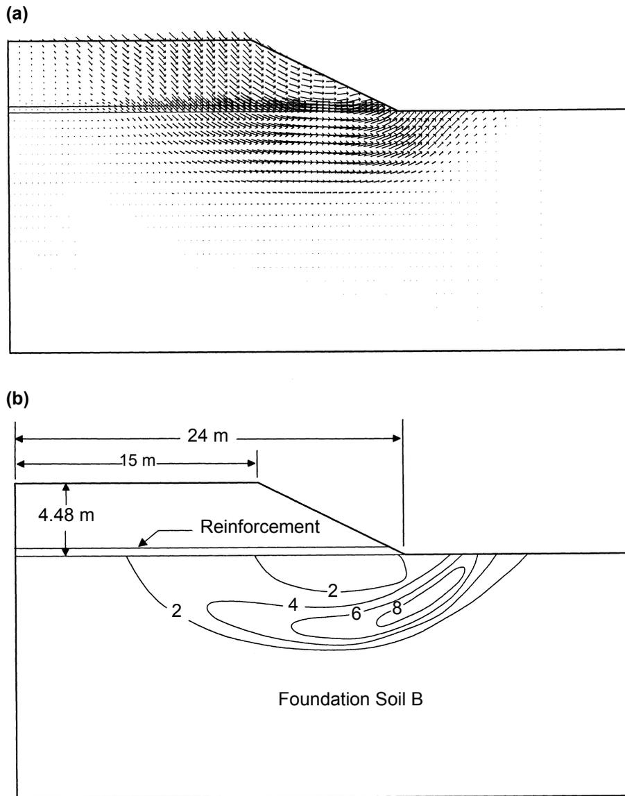
**Figure 13.** Deformations of foundation Soil B due to 2% creep strain and 0.4% tension strain of G1 between the end of construction and 98% consolidation under the 4.48 m-high, G1-reinforced embankment: (a) velocity vector; (b) contours of maximum shear strain (%).
