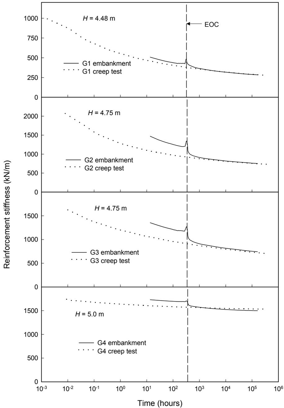
Figure 11. The variation of reinforcement stiffness with time for embankments over Soil B.
