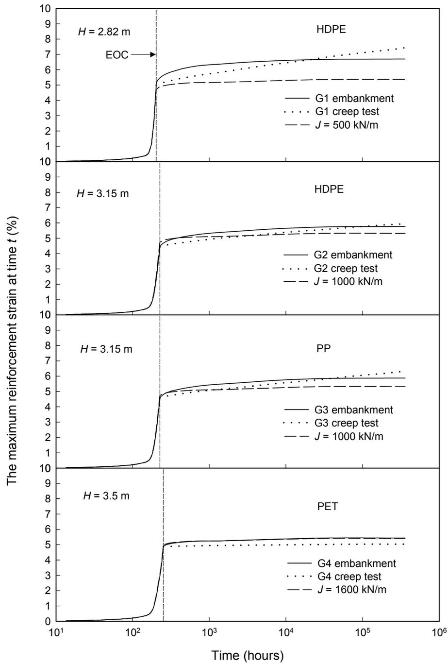
Figure 5. The variation of reinforcement strain with time for embankments over Soil A.
