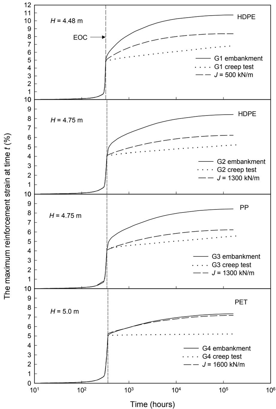
Figure 6. The variation of reinforcement strain with time for embankments over Soil B.
