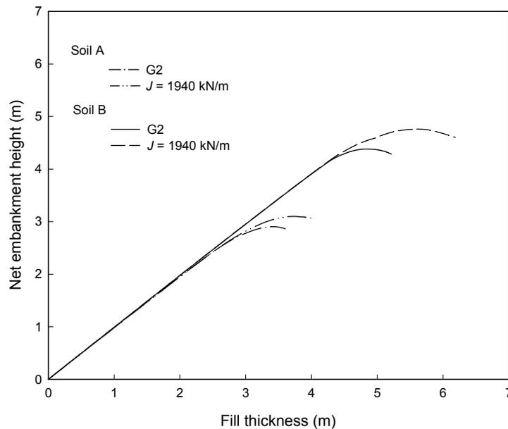
Figure 4. The variation of net embankment height with fill thickness.
