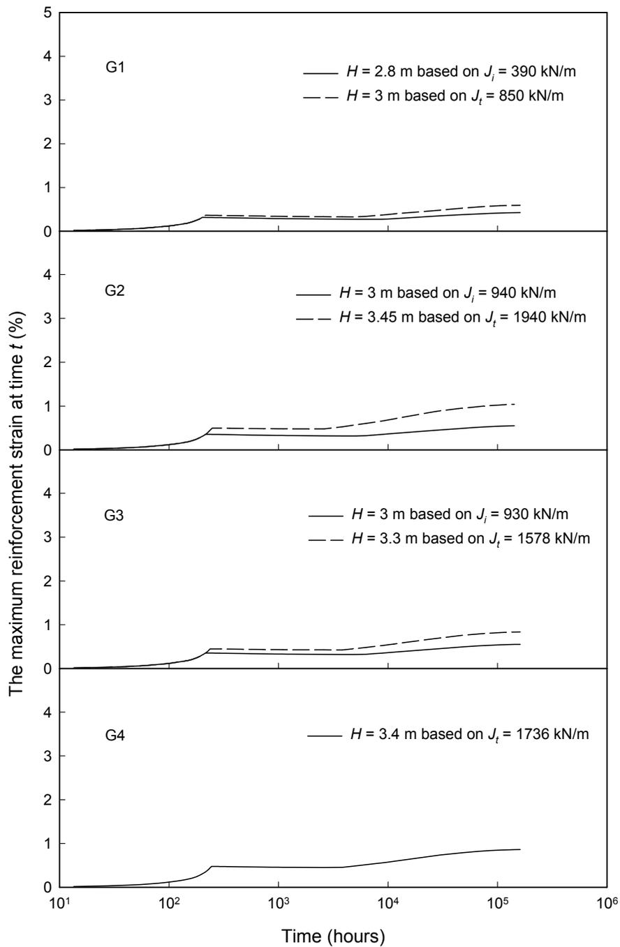
Figure 15. The variation of reinforcement stiffness with time for embankments over Soil B under working conditions.
