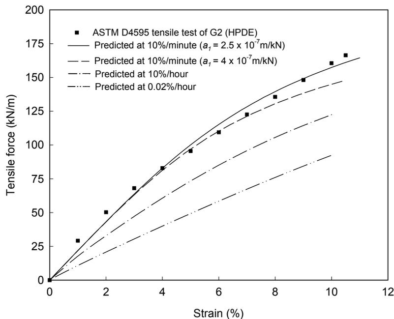
Figure 2. ASTM D 4595 tensile test and predicted results for geosynthetic G2.
