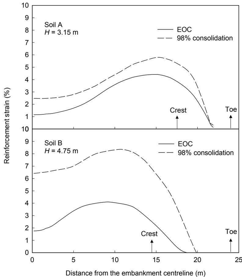
**Figure 7. The distribution of reinforcement strains at the end of construction and 98% consolidation for G2-reinforced embankments over Soils A and B.**
