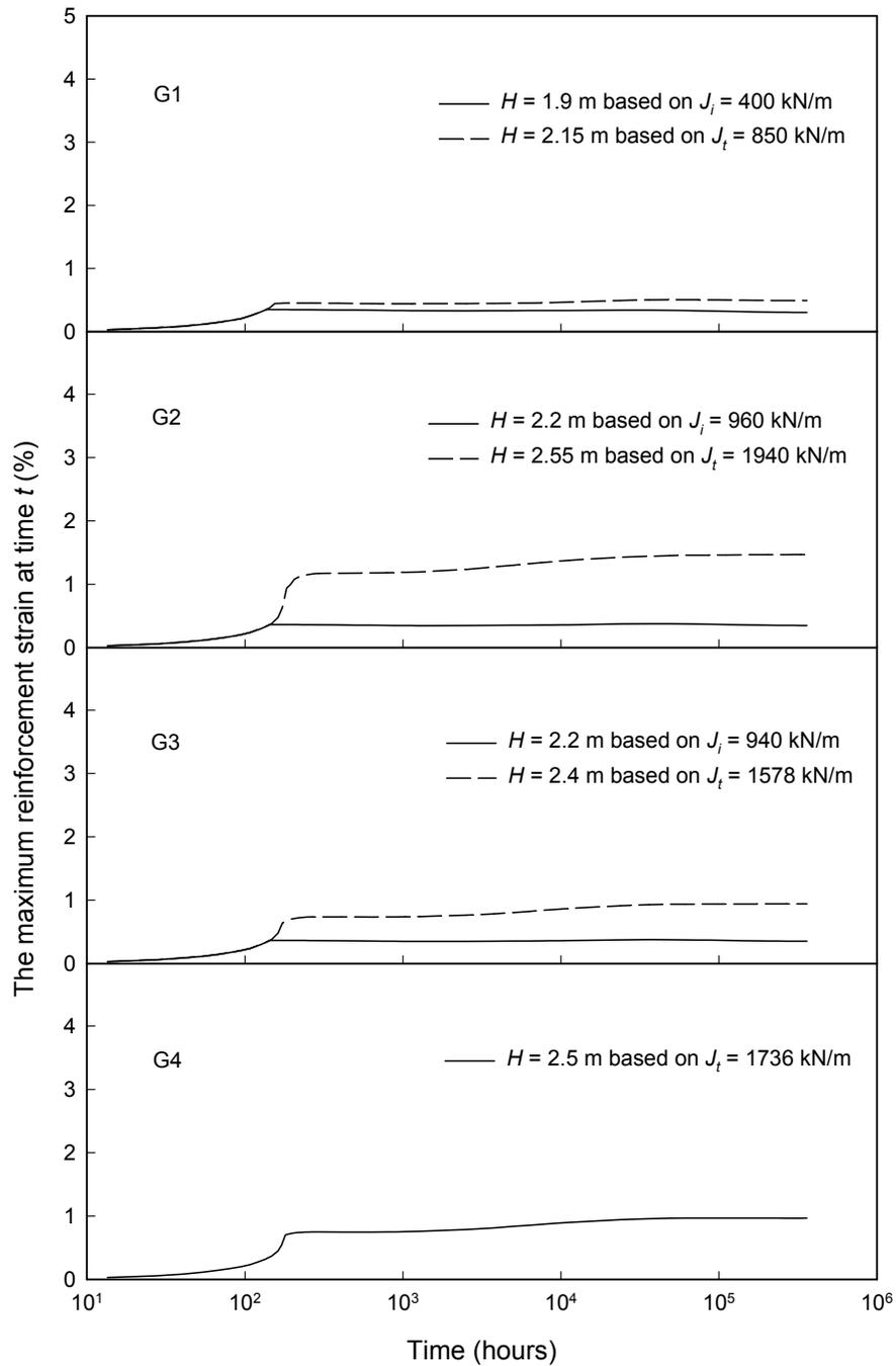
Figure 14. The variation of reinforcement strain with time for embankments over Soil A under working conditions.
