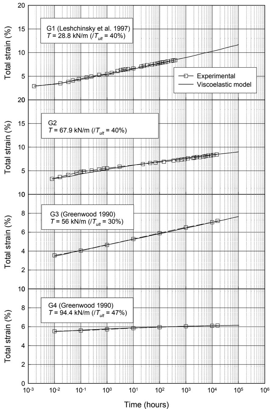
Figure 1. The measured and calculated creep strains of the four geosynthetic reinforcement products.
