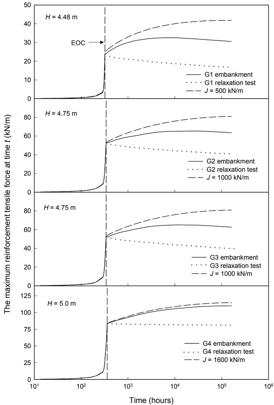
Figure 9. The variation of reinforcement force with time for embankments over Soil B.
