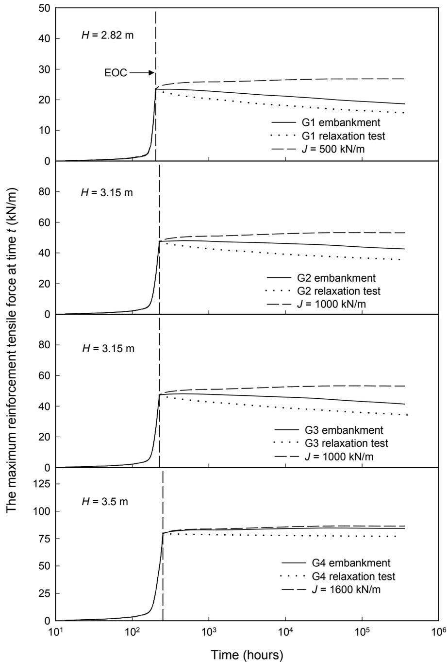
Figure 8. The variation of reinforcement force with time for embankments over Soil A.
