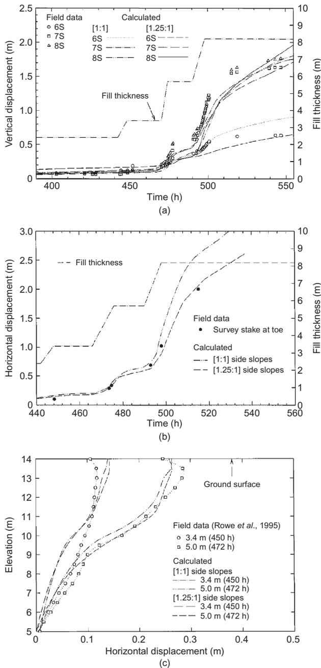
**Figure 7. Comparison of calculated and measured vertical and horizontal deformations (modified from Rowe and Hinchberger 1998): (a) vertical displacement (m) with time (h) at settlement plates; (b) horizontal displacements (m) at embankment toe; (c) relative horizontal displacement profile (m) at inclinometer 231**
