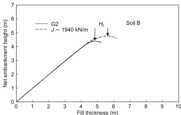
Figure 33. Variation of net embankment height with fill thickness
