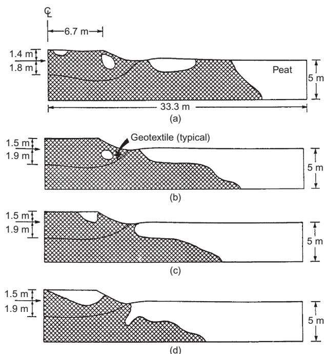
Figure 26. Deformed profile and plastic regions for embankment approximately 1.5 m above original ground level at end of construction,  $B_{\max} = 0.34$ : (a) no reinforcement; (b)  $J = 150$  kN/m; (c)  $J = 500$  kN/m; (d)  $J = 2000$  kN/m (after Rowe and Soderman 1985b)
