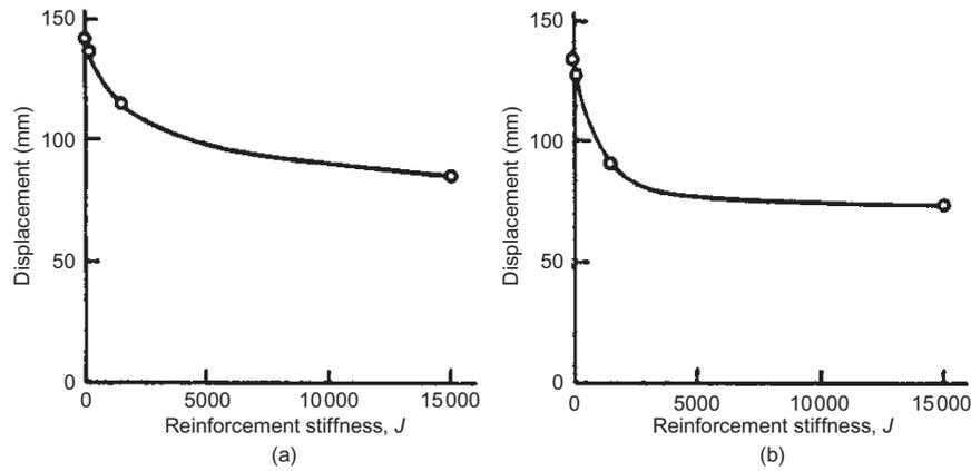
**Figure 8. Effect of reinforcement tensile stiffness,  $J$ , on foundation deformations: (a) maximum settlement of foundation surface; (b) maximum horizontal displacement of foundation surface (after Hird and Kwok 1990)**
