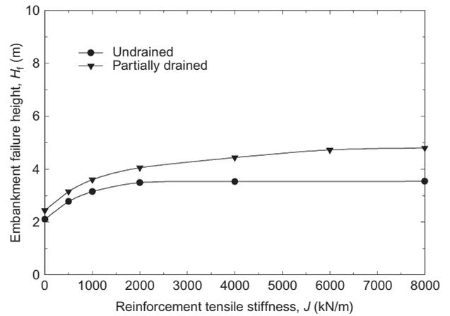
Figure 16. Embankment failure height against reinforcement tensile stiffness
