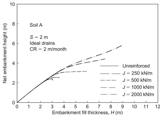
**Figure 20. Variation of net embankment height with fill thickness**
