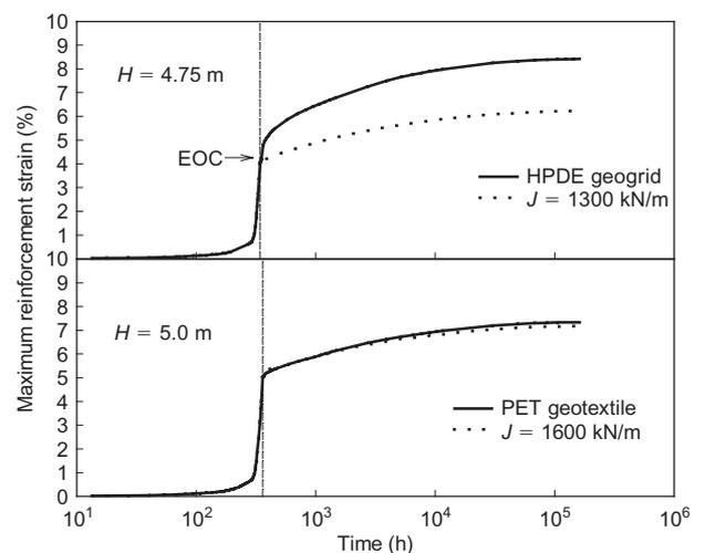
Figure 34. Variation of reinforcement strain with time for embankments over Soil profile B
