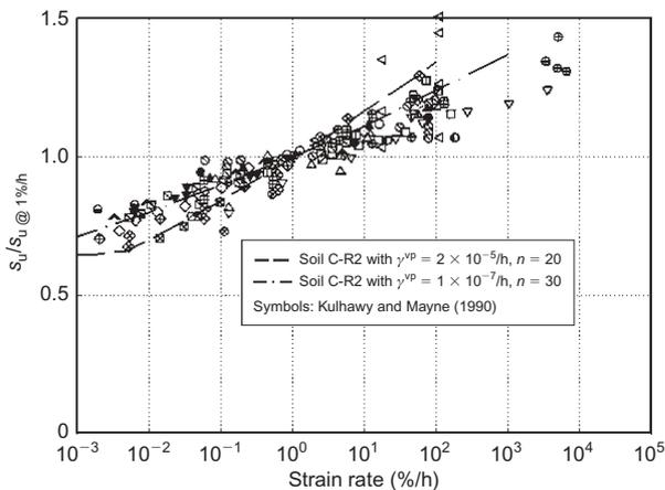
**Figure 28.** Effect of strain rate on undrained shear strength  $s_u$  of Soils C-R1 and C-R2 (after Li and Rowe 2002)
