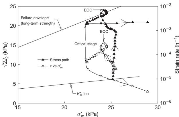
Figure 31. Stress path and strain rate at Point A for 5 m-high reinforced ( $J = 2000 \text{ kN/m}$ ) embankment over Soil C-R1 (CR = 10 m/month;  $J_2 = \text{second stress invariant}$ )
