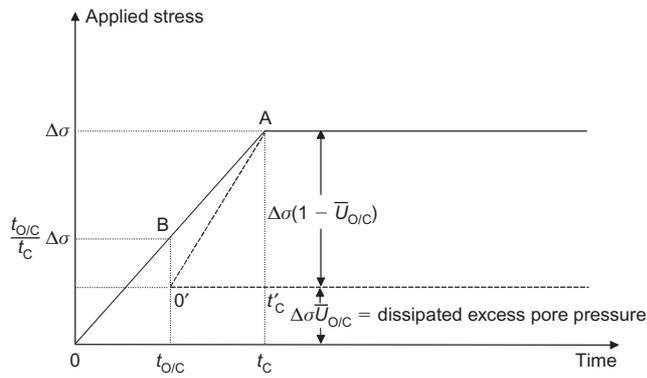
**Figure 24. Breakdown of linear ramp load function for consolidation analysis considering the soil in its overconsolidated and normally consolidated states (modified from Li and Rowe 2001a)**
