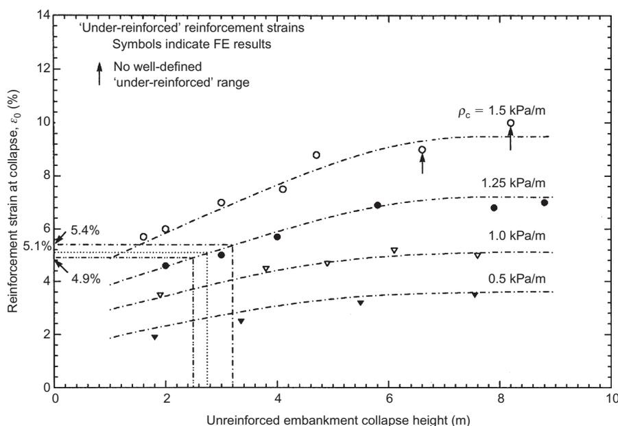
**Figure 14. Chart for estimating reinforcement strains at embankment failure for foundation soils with strength increase with depth (modified from Hinchberger and Rowe 2003). (Note: This chart only considers soil–reinforcement interaction, and the allowable strain may be limited to a lower value by the allowable reinforcement strain based on the strain at rupture)**
