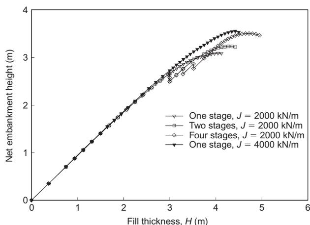
Figure 18. Effect of multi-stage construction on embankment height for Soil profile A
