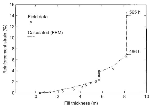
Figure 5. Calculated and measured reinforcement strains against fill thickness (8.8 m from embankment toe) (modified from Rowe and Hinchberger 1998)
