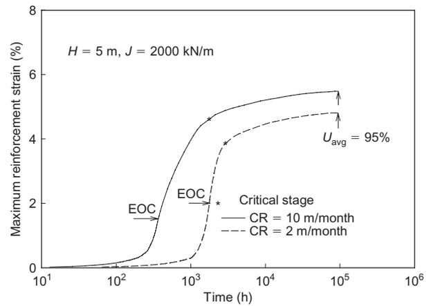
Figure 32. Short-term and long-term reinforcement strains developed for embankments over Soil C-R1
