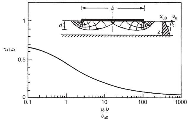
Figure 3. Effect of nonhomogeneity on depth of failure zone beneath a rough rigid footing (modified from Matar and Salencon 1977)
