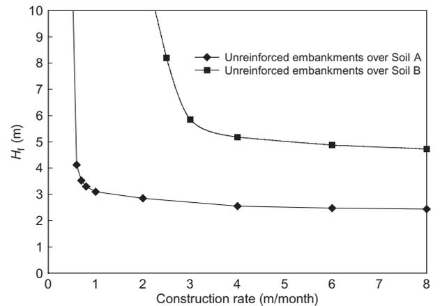
**Figure 22. Effect of construction rate on embankment failure height,  $H_f$  (see Figure 15 for soil profiles)**
