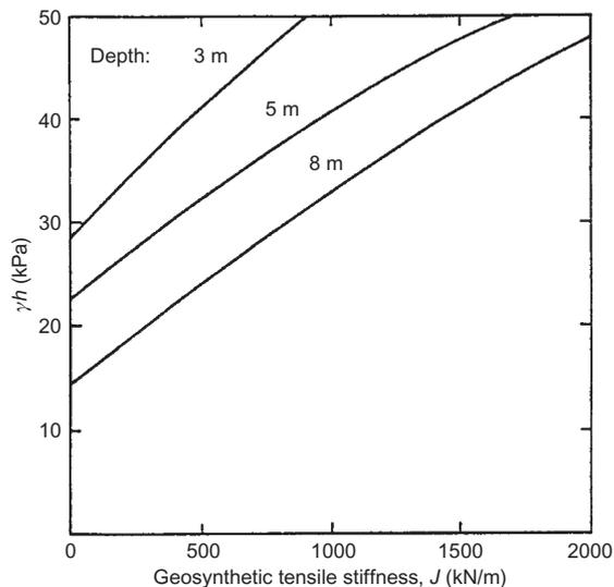
**Figure 27. Design chart for peat underlain by a firm base:**  $B_{\max} = 0.34$ ;  $h$  = height of embankment above original ground level;  $\gamma$  = unit weight of fill (after Rowe and Soderman 1985b)
