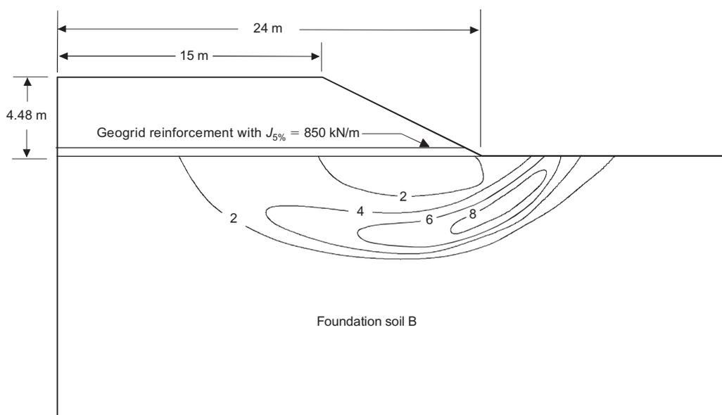
Figure 36. Contours of maximum shear strain (%) in foundation Soil B for 4.5 m-high reinforced embankment due to increase in reinforcement strain of 2.4% between end of construction and 98% consolidation
