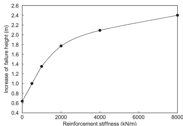
Figure 19. Increase of failure height after 95% consolidation at end of first stage of construction for Soil profile A
