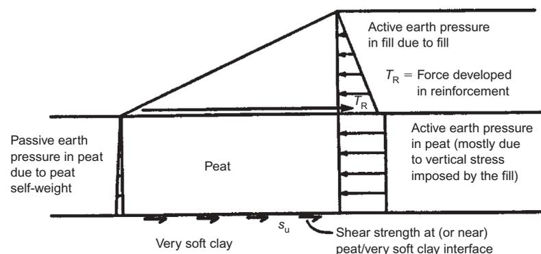
**Figure 25. Potential failure mechanism due to lateral thrust and sliding on a deeper low-strength layer (e.g. very soft clay beneath a peat layer)**
