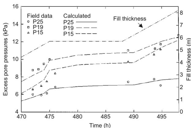
Figure 6. Excess pore pressures at piezometers 15, 19 and 25 during constant embankment loads (5.7 m fill thickness) (modified from Rowe and Hinchberger 1998)
