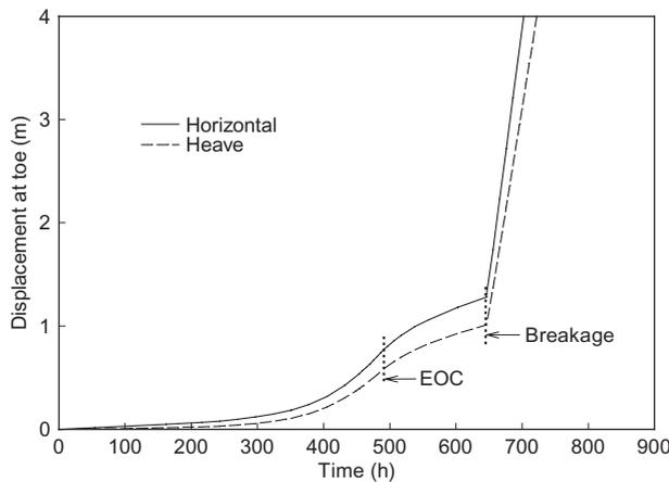
**Figure 30.** Displacements at toe for case with  $J = 2000$  kN/m,  $H = 6.75$  m and reinforcement breaking at  $\epsilon = 10\%$
