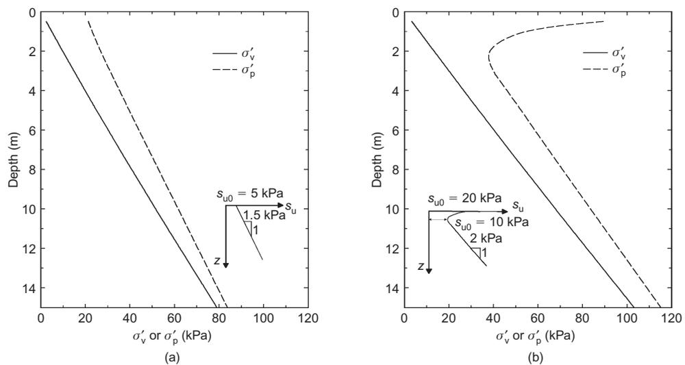
Figure 15. Preconsolidation profiles: (a) foundation soil A; (b) foundation soil B (after Rowe and Li 1999)
