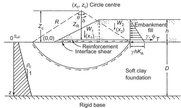
Figure 4. General arrangement of limit equilibrium method by Mylleville and Rowe (1988)
