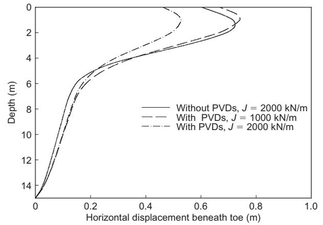
**Figure 21. Comparison of horizontal displacements below toe at end of construction on Soil profile A,  $H = 3.5$  m**
