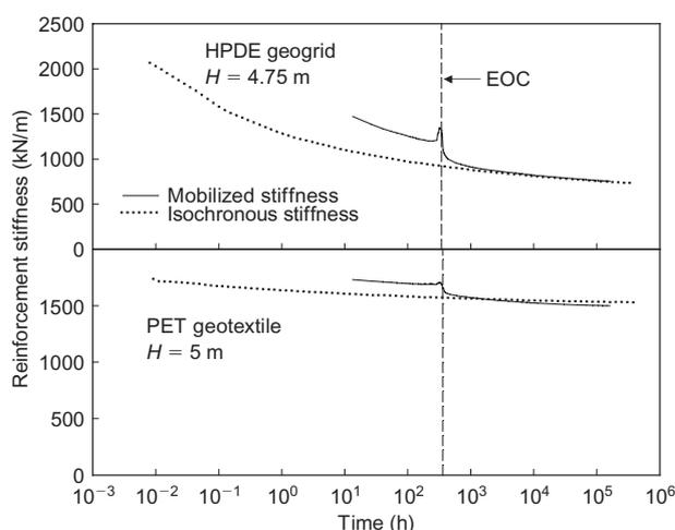
Figure 35. Variation of reinforcement tensile stiffness with time
