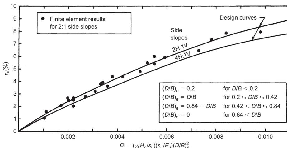
Figure 10. Variation of allowable compatible strain  $\varepsilon_a$  with dimensionless parameter  $\Omega$  modified from Rowe and Soderman 1985a)
