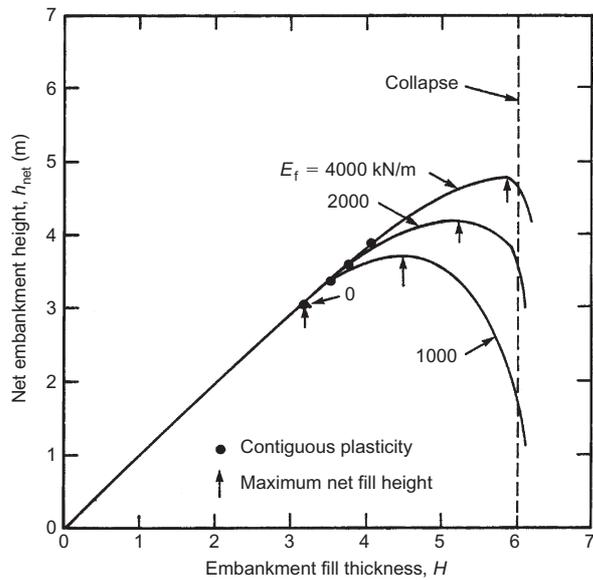
Figure 12. Net embankment height against fill thickness for various reinforcement tensile stiffness values (after Rowe and Soderman 1987b)
