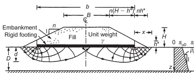
Figure 2. Definition of variables used to estimate collapse height for a perfectly reinforced embankment (modified from Rowe and Soderman 1987a)
