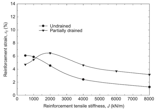
Figure 17. Reinforcement strain at failure (Soil profile A – Figure 15)
