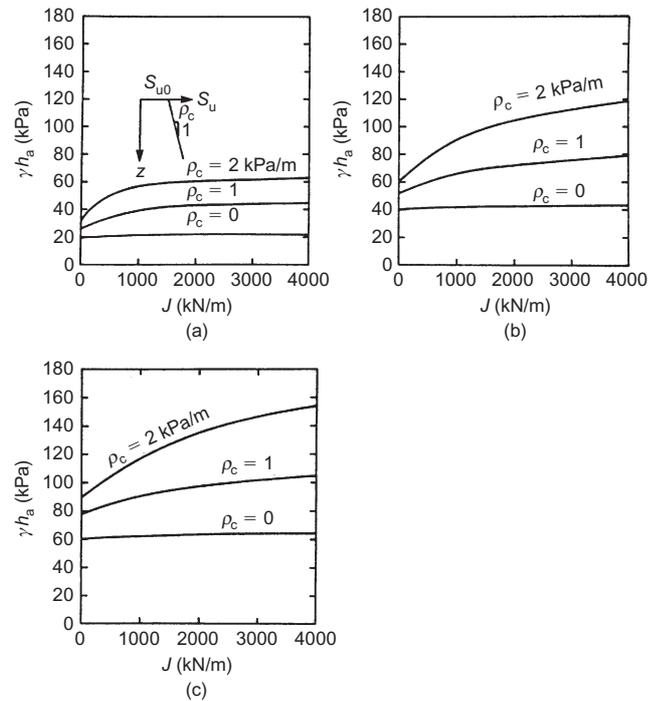
Figure 13. Allowable pressures,  $\gamma/h_a$  (based on FS = 1.3) against tensile stiffness,  $J$ , for different foundation soils, where  $\rho_c$  is rate of increase in undrained shear strength with depth (kPa/m) (modified from Rowe and Soderman 1987b): (a)  $s_{u0} = 5$  kPa, (b)  $s_{u0} = 10$  kPa, (c)  $s_{u0} = 15$  kPa
