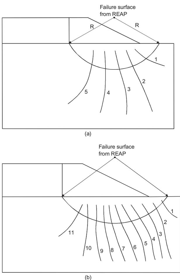
Figure 23. Contours showing increase in undrained shear strength,  $\Delta s_u$  in kPa, at end of construction, from FEM analyses: (a) Soil A, ideal drains,  $S = 2 \text{ m}$ ,  $H = 4.41 \text{ m}$ ,  $CR = 2 \text{ m/month}$ ;  $J = 2000 \text{ kN/m}$ ; (b) Soil B, ideal drains,  $S = 2 \text{ m}$ ,  $H = 6.48 \text{ m}$ ,  $CR = 4 \text{ m/month}$ ;  $J = 2000 \text{ kN/m}$ ; (after Li and Rowe 2001a)
