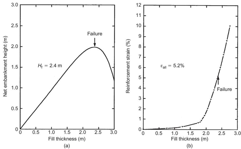
**Figure 9. (a) Maximum net embankment height and (b) allowable reinforcement strain on soil with  $s_{u0} = 3.8$  kPa and  $\rho_c = 1.5$  kPa/m and reinforcement with  $J = 600$  kN/m (after Hinchberger and Rowe 2003)**
