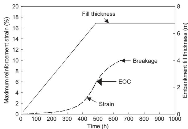
**Figure 29.** Reinforcement strain developed during short-term for embankments with CR = 10 m/month,  $J = 2000$  kN/m over Soil C-R1
