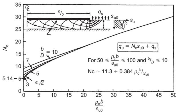
Figure 1. Bearing capacity factor for nonhomogeneous soil (modified from Rowe and Soderman 1987a)
