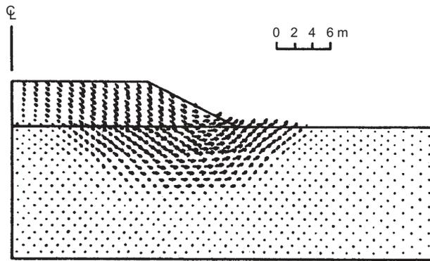
Figure 11. Velocity field at collapse for reinforced embankment ( $J = 4000$  kN/m) on foundation soil with  $s_{u0} = 7.69$  kPa and  $\rho_c = 1.54$  kPa (after Rowe and Soderman 1987b)
