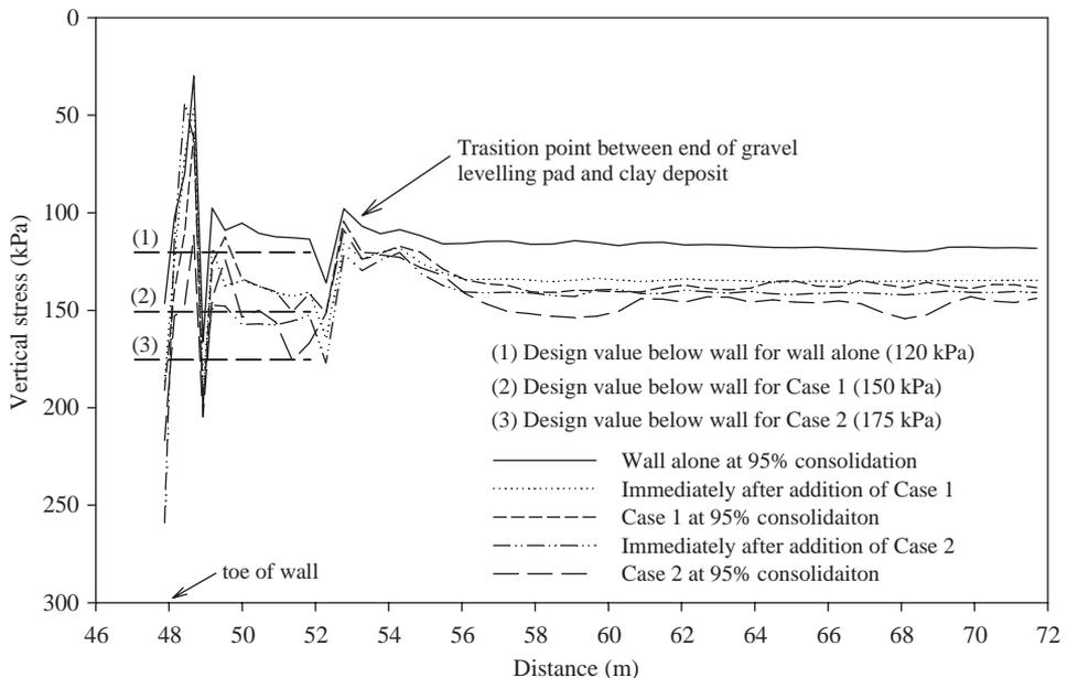
Fig. 10. Vertical stress at base of wall after Cases 1 and 2 loadings were applied and at 95% consolidation (95% consolidation = % degree of consolidation at a point along right lateral boundary at centre of foundation deposit).
