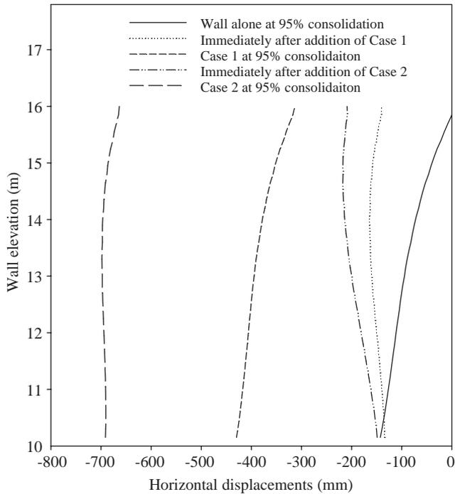
Fig. 8. Horizontal displacements at wall face after Cases 1 and 2 loadings were applied and at 95% consolidation (95% consolidation = % degree of consolidation at a point along right lateral boundary at centre of foundation deposit).
