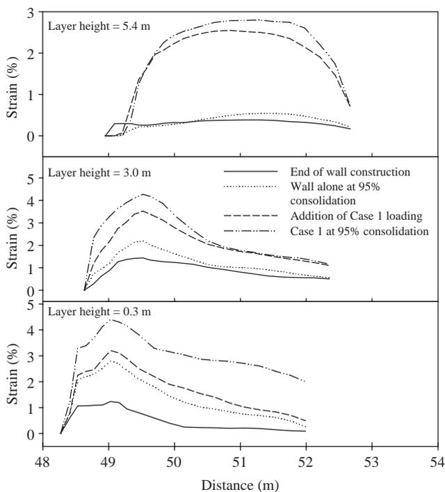
Fig. 12. Strains in various reinforcement layers for Case 1 loading (95% consolidation = % degree of consolidation at a point along right lateral boundary at centre of foundation deposit).
