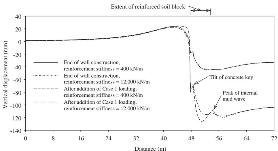
Fig. 15. Vertical displacement at base of wall for extended bottom reinforcement layer with stiffnesses of 400 and 12,000 kN/m.
