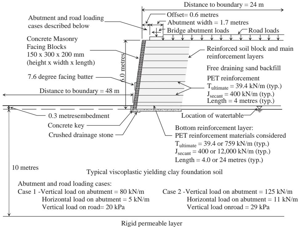
Fig. 1. Cross-section of typical wall with bridge abutment and approach road loads.
