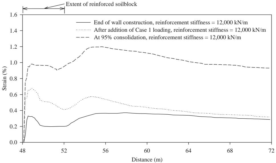
Fig. 16. Strain in extended bottom reinforcement layer with stiffness of 12,000 kN/m (95% consolidation = % degree of consolidation at a point along right lateral boundary at centre of foundation deposit).
