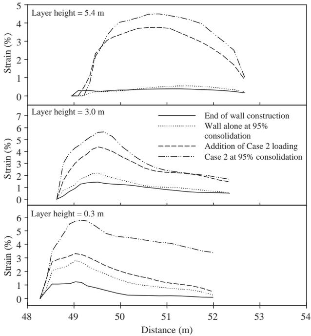
Fig. 13. Strains in various reinforcement layers for Case 2 loading (95% consolidation = % degree of consolidation at a point along right lateral boundary at centre of foundation deposit).
