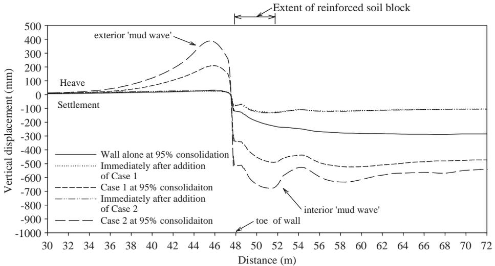
Fig. 9. Vertical displacements at base of wall after Cases 1 and 2 loadings were applied and at 95% consolidation (95% consolidation = % degree of consolidation at a point along right lateral boundary at centre of foundation deposit).
