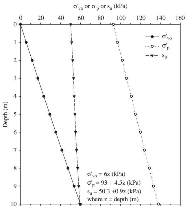
Fig. 3. Initial effective stress, preconsolidation pressure and undrained shear strength of clay foundation soil ( $s_u$  = Bjerrum (1973) corrected shear vane strength).
