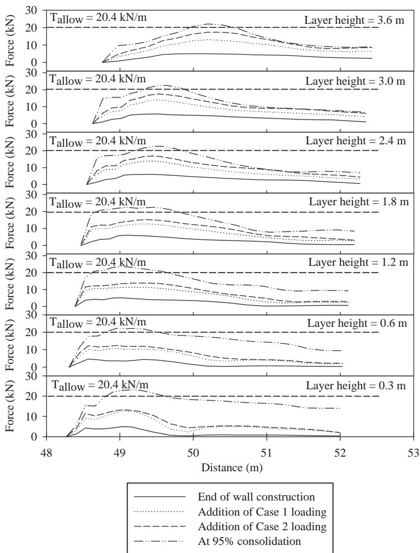
Fig. 14. Forces in reinforcement layers below 3.6m height for Case 2 loading (95% consolidation = % degree of consolidation at a point along right lateral boundary at centre of foundation deposit).
