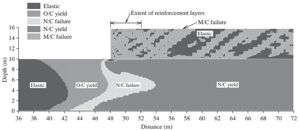
Fig. 5. Plasticity zones in wall and foundation after Case 1 loading applied.
