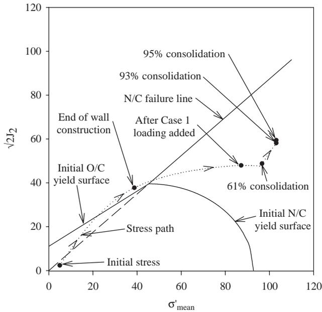
Fig. 4. Stress path at a point 1 m below toe of wall for Case 1 loading.
