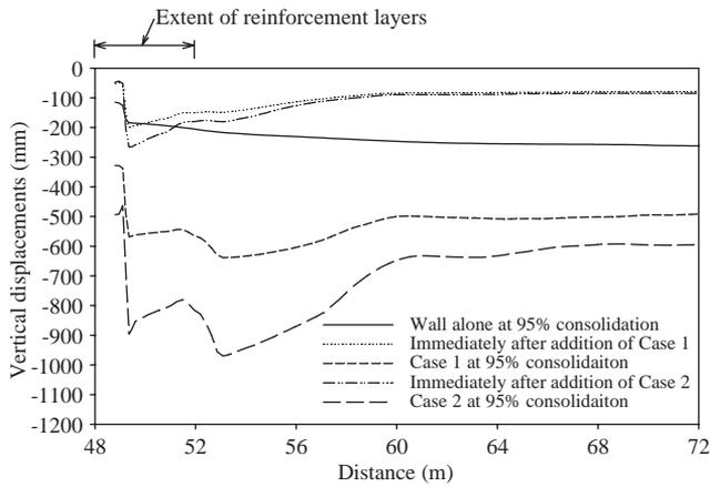
Fig. 7. Vertical displacements at top of wall after Cases 1 and 2 loadings were applied and at 95% consolidation (95% consolidation = % degree of consolidation at a point along right lateral boundary at centre of foundation deposit).
