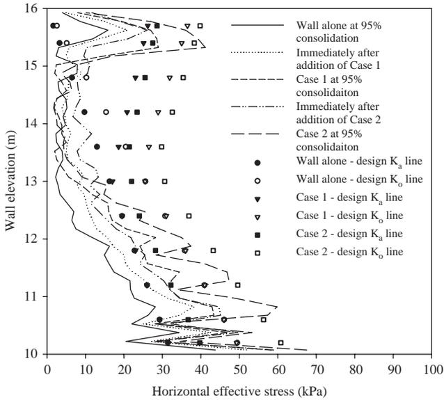
Fig. 11. Horizontal effective stress along back of wall face after Cases 1 and 2 loadings were applied and at 95% consolidation (95% consolidation = % degree of consolidation at a point along right lateral boundary at centre of foundation deposit).
